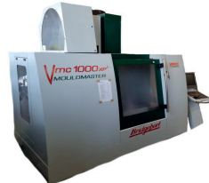
Bridgeport VMC 1000xp2 (x-axis 1020 mm, y-axis 610 mm, z-axis 610 mm, work table 1150x580 mm)
