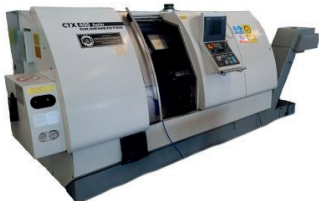
Gildemeister CTX 400 TWIN (max Ø 250 mm, two heads, with material feeder max 65mm and 1500mm long, xyz 220x635x80(+/-40mm) mm)
