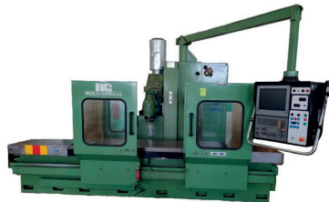
Nc Calidad Correa cf2 (x-axis 2500mm, y-axis 800mm, z-axis 800 mm, work table 2535x700 mm)
